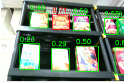
Figure 4.8: A sample product detection result that was robust to blurring and overexposure with the help of data association .
