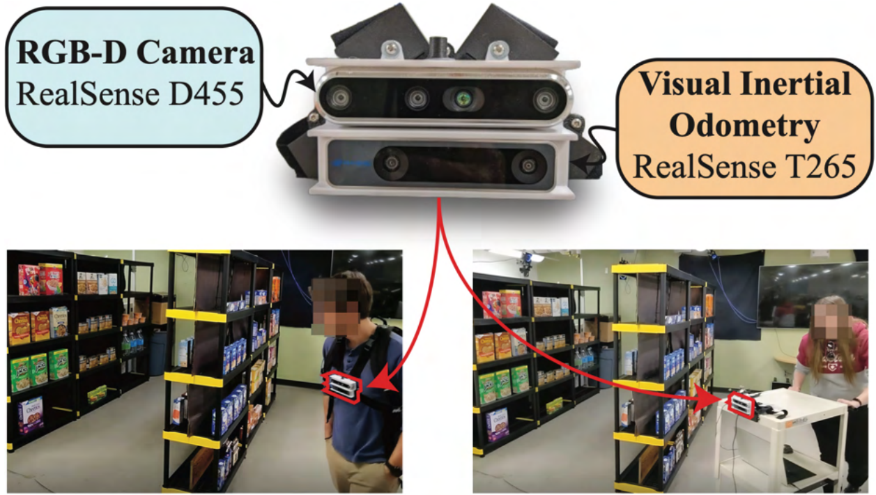
Figure 5.5: ShelfAware hardware. A lightweight two-camera system with a 3D-printed mount was used throughout our experiments (top). This design allowed evaluation across a wearable chest mount (left) and a cart-mounted setup (right).
