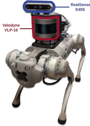
Figure 6.3: Go1 with RealSense D455 and Velodyne VLP-16.
